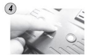
Step 4: Press and hold (2 seconds) UIS On/Off button to activate internet protection.
