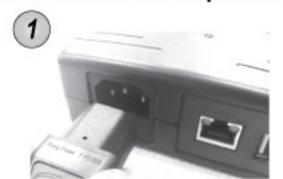
Step 1: Connect the power cord to device and wall outlet.
