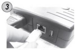
Step 3: Connect LAN cable from Router. The Internet LED will turn ON to indicate online.
